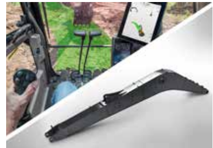
Long Reach boom & arm with Dig Assist
