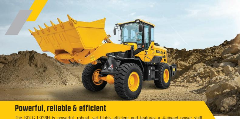
The SDLG L938H is powerful, robust, yet highly efficient and features a 4-speed power shift transmission for smoother shifting and greater speed capabilities. The L938H is the ideal machine for transporting and loading loose materials, general material handling, and construction work with an extensive range of attachments available for ultimate versatility and productivity.
